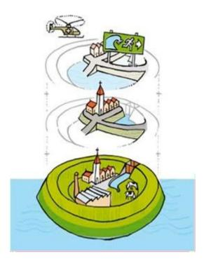
Multi-layer safety is based on a risk approach: the focus is on both the probabilities and the possible consequences of flooding. The first layer is *prevention*: trying to prevent floods as much as possible. Measures to reduce the *impact* of a flood are found in layers 2 and 3. The second layer focuses on structuring our country on water-robust lines. The third layer is about good disaster management.
