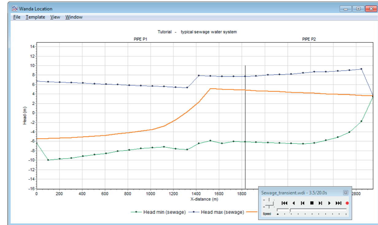
Analysis of pressure wave propagation through a pipeline
