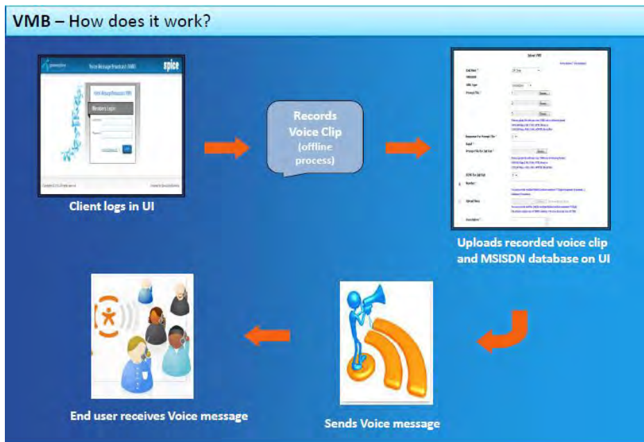
Figure 4.2 Overview of how the Voice Message Broadcast (VMB) works
