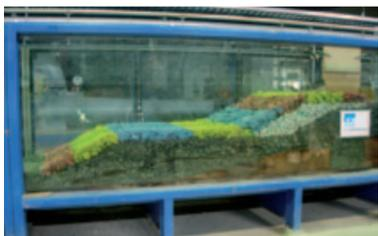
The design of several breakwaters for the protection of the Dubai coastal developments against severe wave attack was tested by means of scale tests in our facilities. In these tests the stability of armour layers and the amount of wave overtopping for different design alternatives were quantified under a series of severe storm conditions. Based on the results of the scale tests, the designs were validated or optimised.
